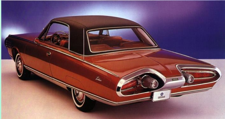
Chrysler “Turbine” (1963) – turboshaft powered consumer vehicle.
